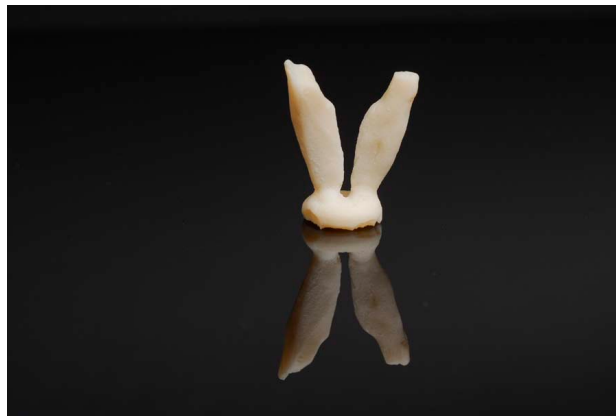
Fig. 4. Ceramic phantom prior to embedding in acrylic base
