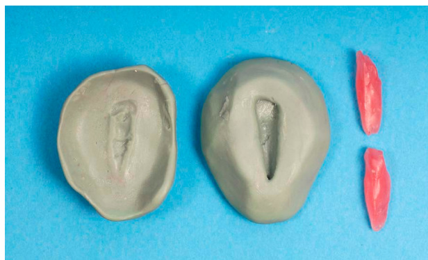
Fig. 2. Silicone matrix and wax patterns for preparing ceramic phantoms
