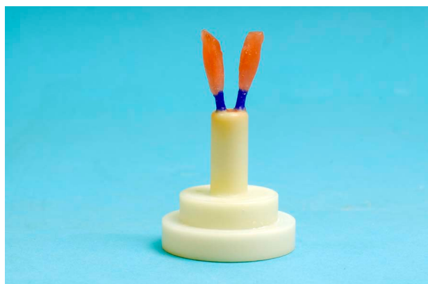
Fig. 3. Wax patterns embedded on casting cone
