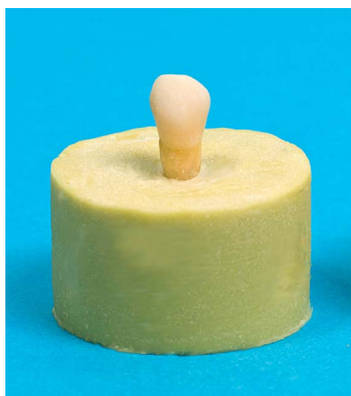
Fig. 1. Tooth embedded in an acrylic block
