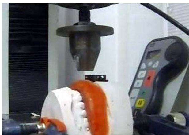
Fig. 4. Mouthguard in MTS Q/Test 10 device
